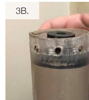
4. Clean any remaining clay from the tube and its apertures with a sponge and the wire brushes in a 5-gallon bucket in the dry sink.
