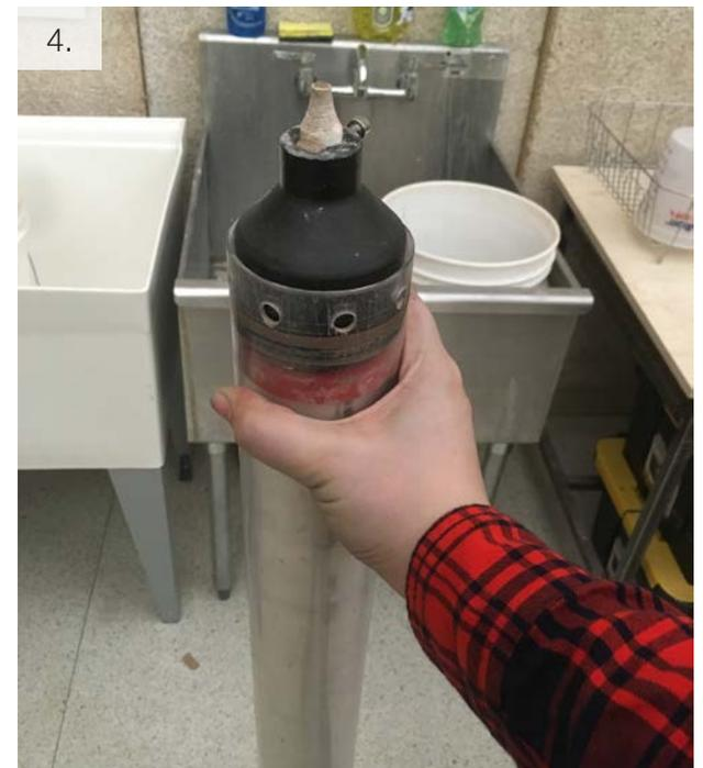
5. Separate the nozzle holder from the extruder piece
